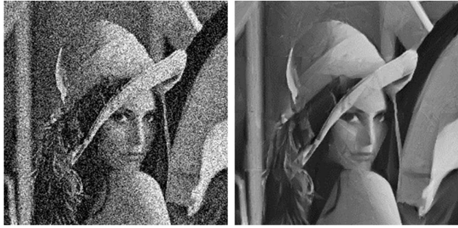
(a) Noisy PSNR=16.57 dB. (b) De-noised PSNR=26.4 dB.
