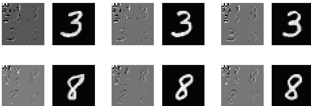
FIGURE 8. Digits generated with Top- p = 0.6 along with a depiction of the generated wavelet coefficients.
